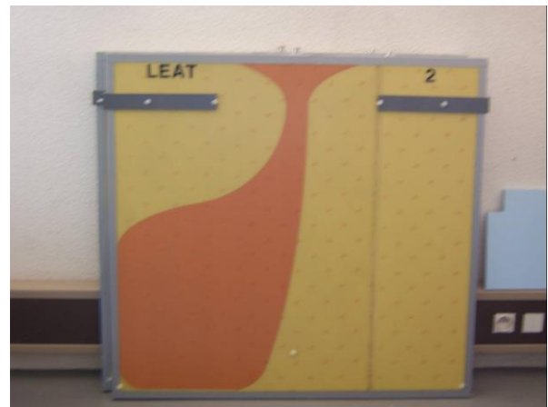
Fig. 1: ETSA antenna with exterior ground plane visible.
