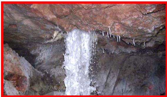
Fig. 1 Water infiltrating an underground potash mine in Saskatchewan.
