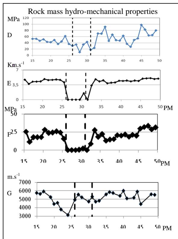
Figure 1 : Rock mass rock physical properties across the fault zone (A) faulting degree (RQD); (B) joints roughness (JRC); joint alteration here no filling or clay (Ja); (C): micro-porosity evolution and relationship with the micro-cracks; (D) uniaxial compressive strength; (E)  $V_p$  for rock mass; (F) Young modulus rock mass, (G)  $V_p$  on sample.
