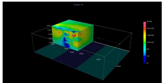
Fig. 4 3D inverse model sliced to highlight low resistivity/high porosity zone viewed from nominal NE direction.
