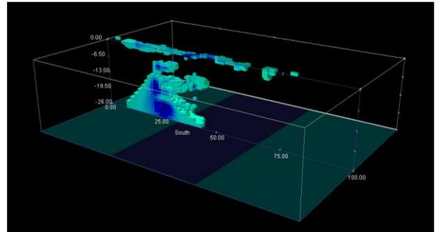
Fig. 3 3D inverse model with iso-surface cutoff highlighting low resistivity zones. Deeper structure is poorly constrained on the bottom face.
