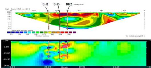
Fig. 2 Comparison of 2D (upper) inversion of Wenner-Schlumberger data and 3D inversion of complete data set on similar plane with borehole televiewer data overlaid.
