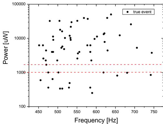
FIG. 2: scatter plot of power and primary frequency of the 61 true events, with the gap around  $10^3 \mu\text{W}$  demarcating the high ( $\alpha$ ) from the low (neutron) amplitude populations.
