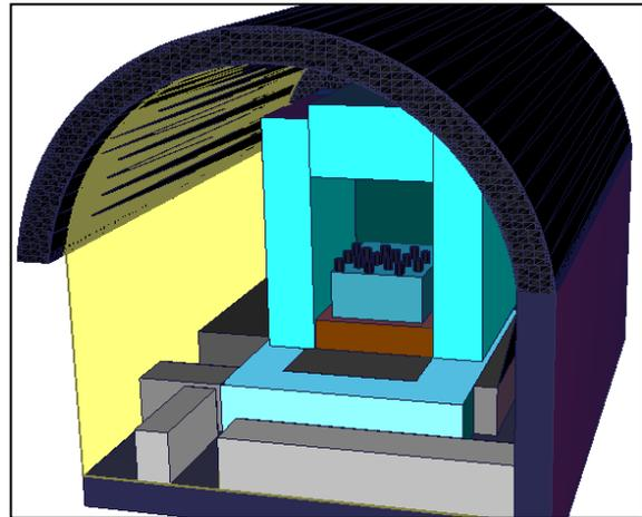
Fig. 1: schematic of the SIMPLE SDDS in the GESA site. The dark areas represent wall concrete, the light areas, the floor concrete and water shield surrounding the centrally located detectors.
